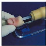
Thread the flexible plastic strip attached to the toe through the slot at the front of the spindle on the toe jig.
